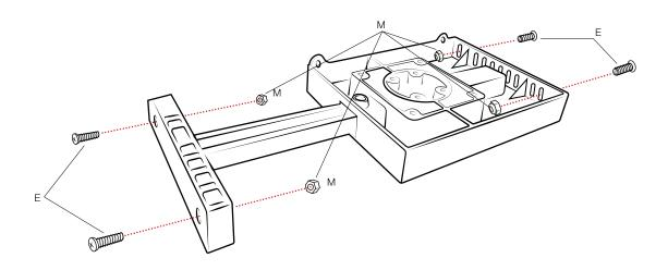
6 Use (F) screws and rest of (M) nuts to attach RAM® Tough-Tray™ to any RAM® Mount.
